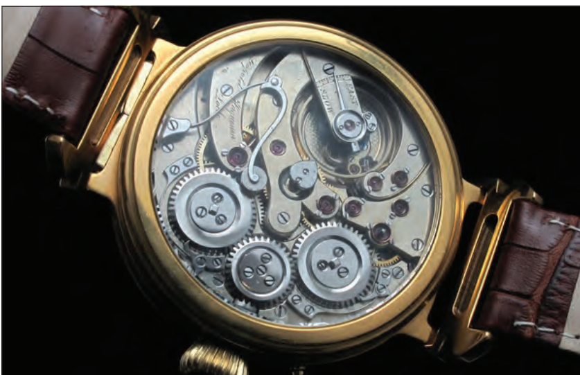
Figure 2. Back of the Léopold Huguenin watch, serial number 12987. Note the seven jewels with screwed-in gold settings. Both spring barrels are wound simultaneously via the crown.
