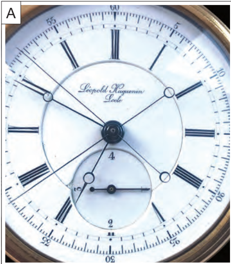
Figure 1. A , Léopold Huguenin former pocket watch, re-cased as a 'marriage watch', showing the sweep-seconds hands which are part of the split-seconds system; and the jump quarter-seconds hand and subsidiary dial at the VI position on the three-piece enamel dial. B , behind the dial of A , with the minute and hour wheels removed to expose the jump quarter-seconds flirt, and the serial number 12987 (cropped). a one of the four tines on the flirt; b cock with the flirt arbor jewel and the jewel for the fifth wheel arbor of the jump quarter-seconds train; c flirt arbor that carries the jumping hand; d spotted mainspring barrel cap of the jump quarter-seconds train; e barrel cap of the going train; f clutch (a steel bush) and 40-tooth wheel mounted on the extension of the third-wheel arbor of the going train; this wheel engages with the adjacent 40-tooth wheel seen here, and also with a third 40-tooth wheel (not shown) that rides over the post of the minute hand. The eight-leaf pinion on the second 40-tooth wheel engages with a 96-tooth hour wheel (not shown); C , behind the dial of the movement bought at Rikketik, serial number 13728 (cropped).
